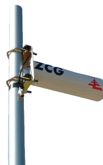
Y2400-9 installed onto pole in correct orientation with drain hole facing down, allowing any humidity ingress to expell
