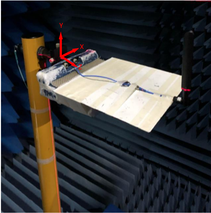
Bent 30x30cm Ground Plane Edge
